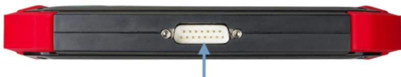
DB15 Port: Connect to the main test cable
