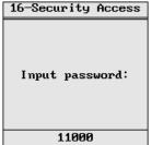
Press left/right button to choose number of places. Press up/down button to enter the passing code and then press [Enter]. The following will be
