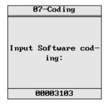
Press Left or Right key to choose the number of places; by Up or Down key to input number. Press [Enter] button to confirm.
