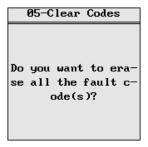
You need to press [Enter] button for the second time to perform "code erase". Of course you can also press [Esc] button to give u. If code erasing successfully, it will display as the following.
