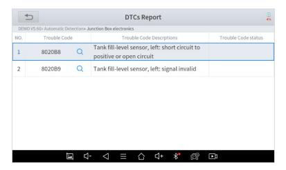
In the process of diagnosis, if the device shows "System is OK" or "No Trouble Code", it means there is no related trouble code stored in ECU or some troubles are not under the control of ECU. Most troubles are mechanical system troubles or executive circuit troubles. It is also possible that the signal of a sensor may be inaccurate but within limits, which can be examined using Live Data.
