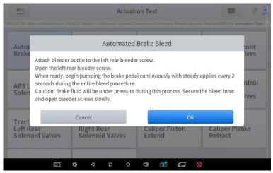
4. When ready, click "*OK*" to enter the bleed procedure, and pumping the brake pedal continuously with steady applies every 2 seconds during the entire procedure
