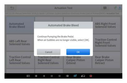
5. Continue pumping the brake pedal, when air bubbles are no longer visible, select **OK** to enter next bleed procedure for left front wheel
