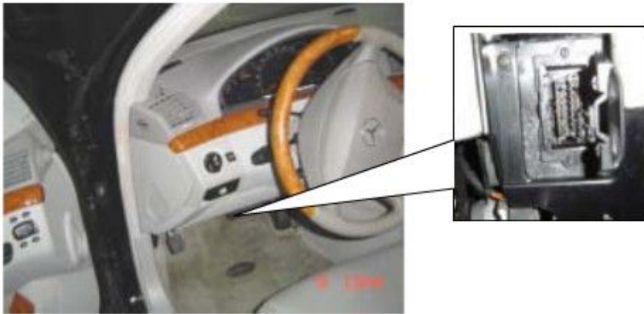
*Benz S320,220 Chassis: the OBD plug is below the dashboard, use SMART OBDII-16 connector.
