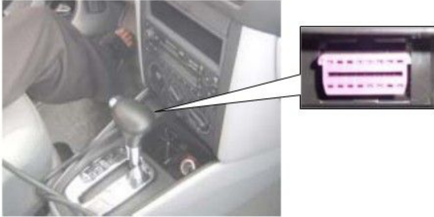
*VW Bollywood 1.8: the OBD plug is below the console, use SMART OBDII-16 connector.
